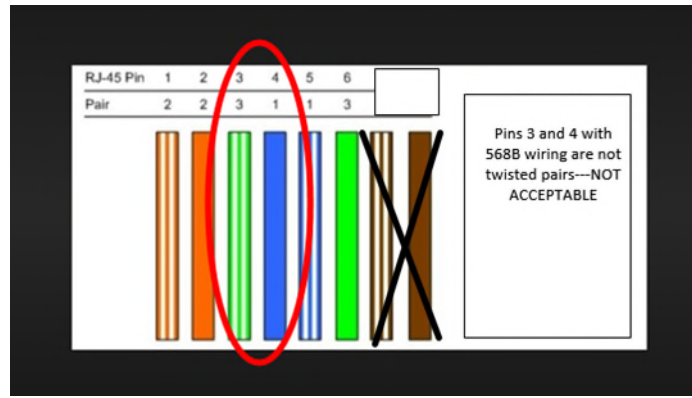
Figure 5 Why Not to Use 568B Wiring-Middle two wires are not a twisted pair!!!!
