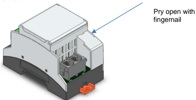
Remove the small plastic shroud on this controller using your finger nail in the top slot of the shroud (see Figure above) and depress and hold the **Discovery Button** for four (4) complete flash cycles (i.e. LED cycles **OFF** immediately, then turns **ON** 1<sup>st</sup> time, then a **LONG OFF**, turns **ON** 2<sup>nd</sup> time, then a **LONG OFF**, then turns **ON** 3<sup>rd</sup> time, then a **LONG OFF**, then when turns **ON** 4<sup>th</sup> time, quickly release
