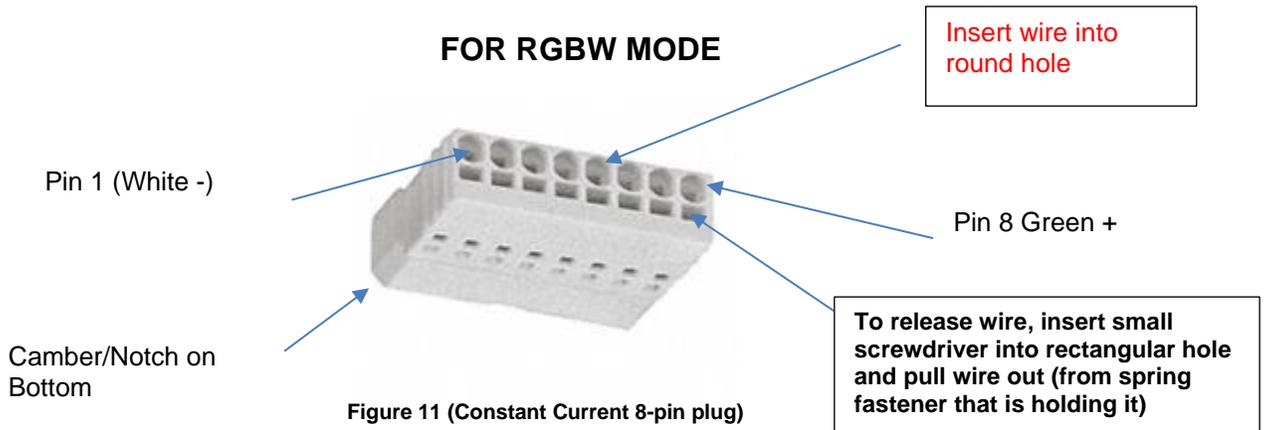
Figure 11 (Constant Current 8-pin plug)
