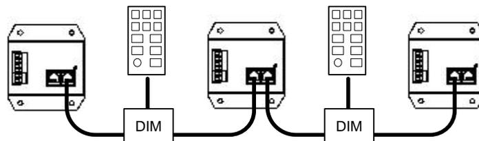
Figure 23 (Multi-DIM devices)
