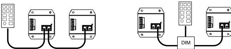
Figure 22 (CS-Bus Wiring)
