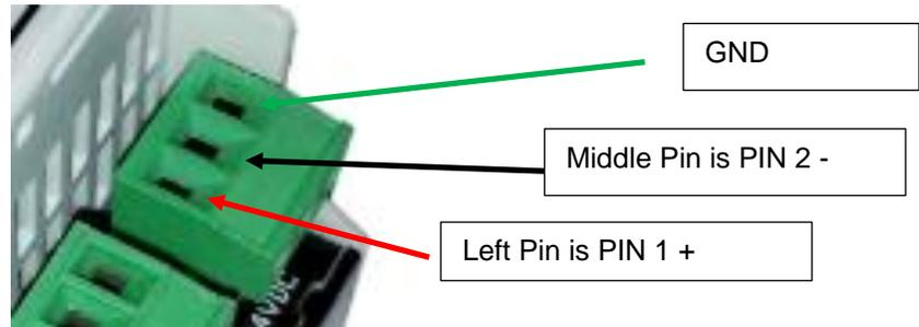
Figure 3 (3-pin power connection)
