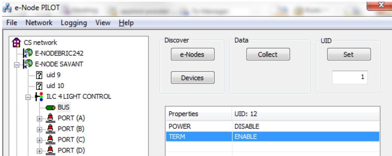
**2. Directions for Turning OFF the Built-in Terminating Resistor on the ILC-400x**
