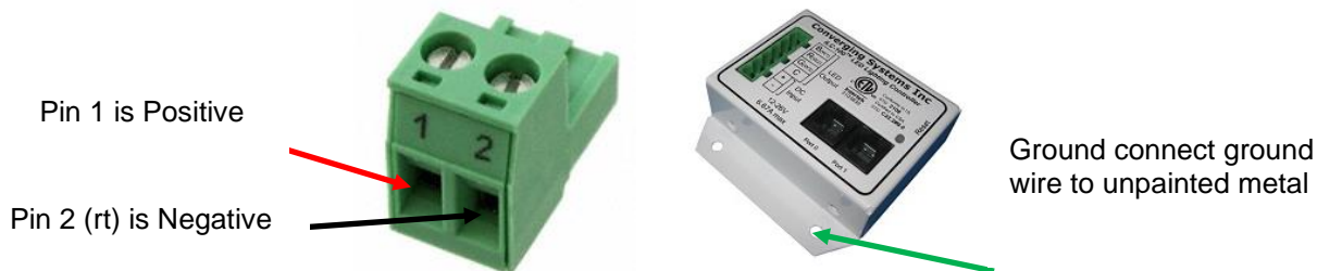
Figure 4 (2-pin power connection w/ chassis ground)
