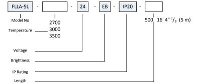
Ordering Example: **FLLA - 5L - 2700 - 24 - EB - IP20 - 500**  *One section 16' 4" long (5 meters), 2700K CCT*
