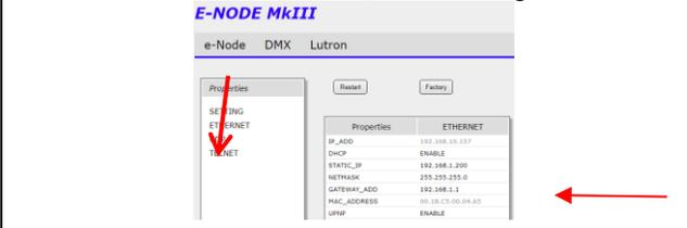
**e-Node Network Parameters.** By default, the e-Node is set to **DHCP ENABLED**. To change to a Static IP address, select the **e-Node** tab to reveal the above setup screen. Select the **ETHERNET** tab and enter a static IP address under **STATIC\_IP**. Then, enter gateway IP address under **GATEWAY\_ADD**. Next, select **DHCP DISABLED** and hit **Restart** to reboot the e-Node to establish the new parameters.
