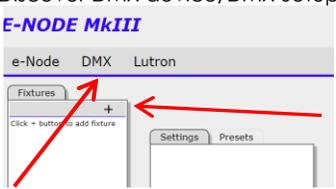
**Add (DMX) Devices.** Select the DMX tab. Click on the + button to add each DMX fixture (up to 32 per e-Node/dmx). Initially, just add all fixtures and later (in Steps 6, and 7) customize those fixtures.
