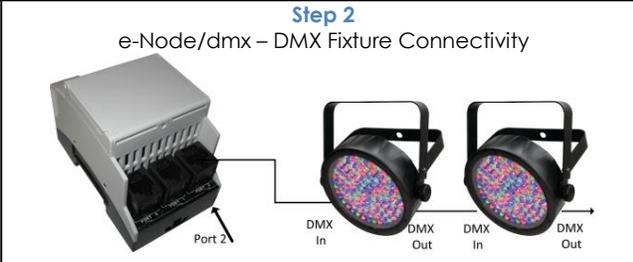
**DMX Fixture wiring.** Port 1 or 2 on the e-Node/dmx is used for data connection to the first DMX fixtures. Additional fixtures should be daisy-chained to the first fixture (max 32 fixtures on chain). Consult the table below for creating your own RJ-45 to DMX Fixture cable (cable not supplied).
