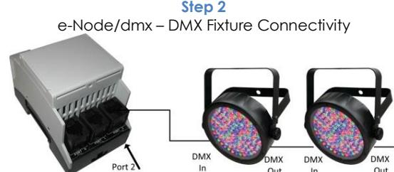
**DMX Fixture wiring.** Port 1 or 2 on the e-Node/dmx is used for data connection to the first DMX fixtures. Additional fixtures should be daisy-chained to the first fixture (max 32 fixtures on chain). Consult the table below for creating your own RJ-45 to DMX Fixture cable (cable not supplied).
