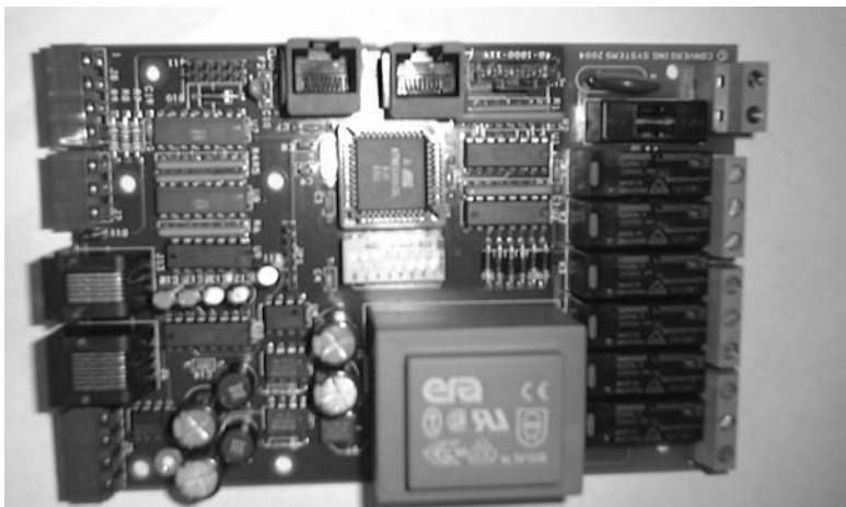
Figure 13. Internal layout of the BRIC circuit board
